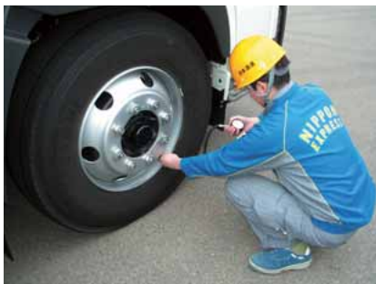
Air pressure measurement using tyre gauge
