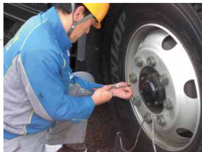
Air pressure measurement using pen-type tyre gauge
