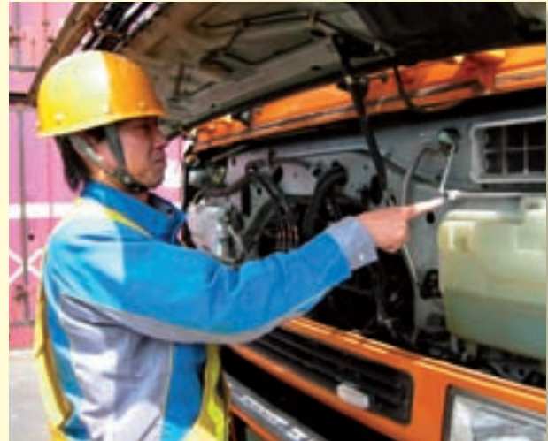
Air-conditioner gas status check using sight glass
